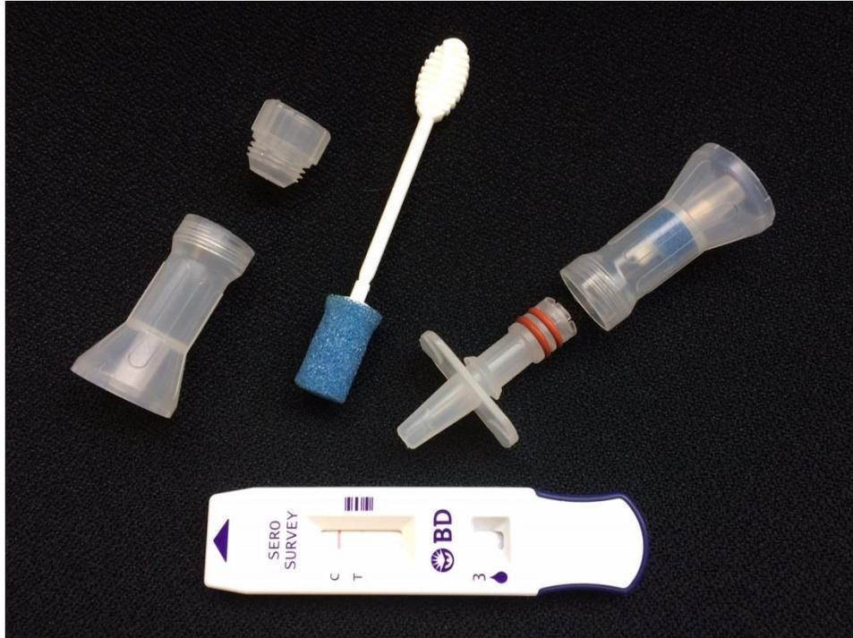
BD-Symbient device to extract oral fluid, mix it with buffer and dispense 3 drops into a BD Veritor™ System cassette
